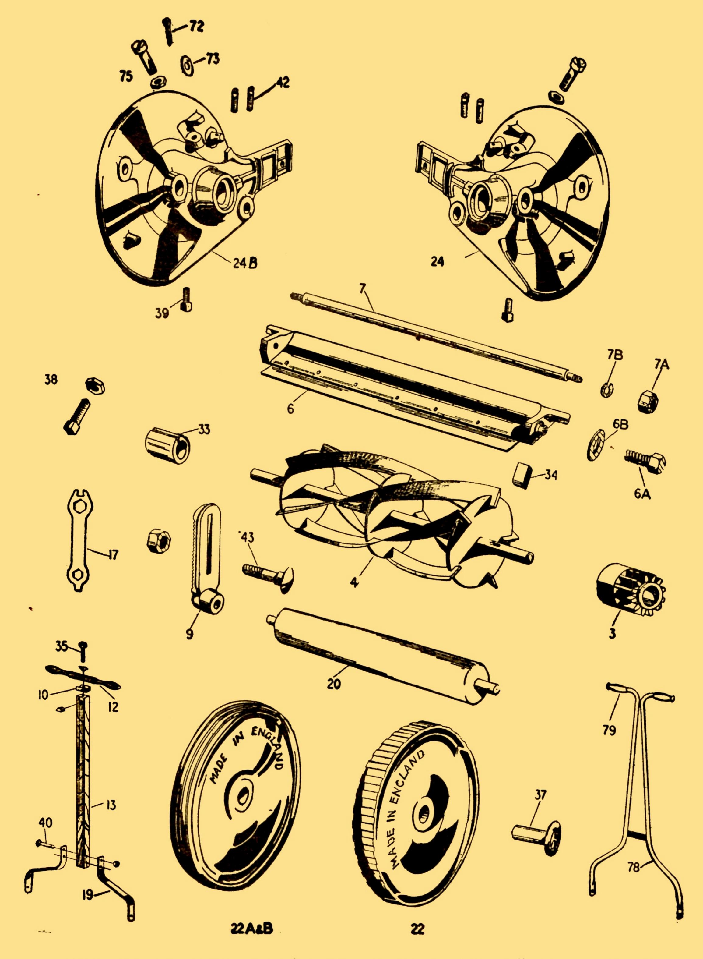
When ordering, please quote the Part Numbers prefixed "L"—not the Diagram Numbers—and state the colour of the part required. Certain parts such as Pinions and Sideplates are made both LEFT HAND and RIGHT HAND. Make sure that you correctly order either L.H. or R.H.
