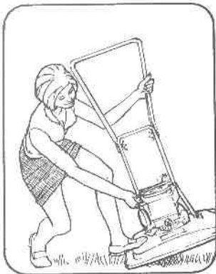
When operating on lawn, remember to tilt the Flymo before switching off. Failure to do this will cause the blade to cut a ring on the lawn.
