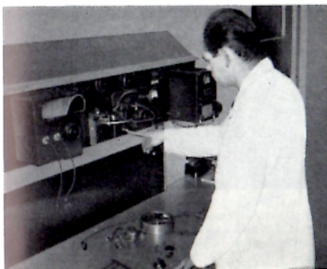
An expert checks the efficiency of a flywheel magneto on a special test rig.
