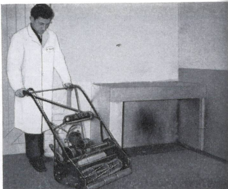
The final running tests are carried out in an air conditioned cubicle where an extractor fan carries the harmful exhaust fumes beyond the factory walls. From here the passed out machine is loaded on to Atco transport for delivery to the User.
