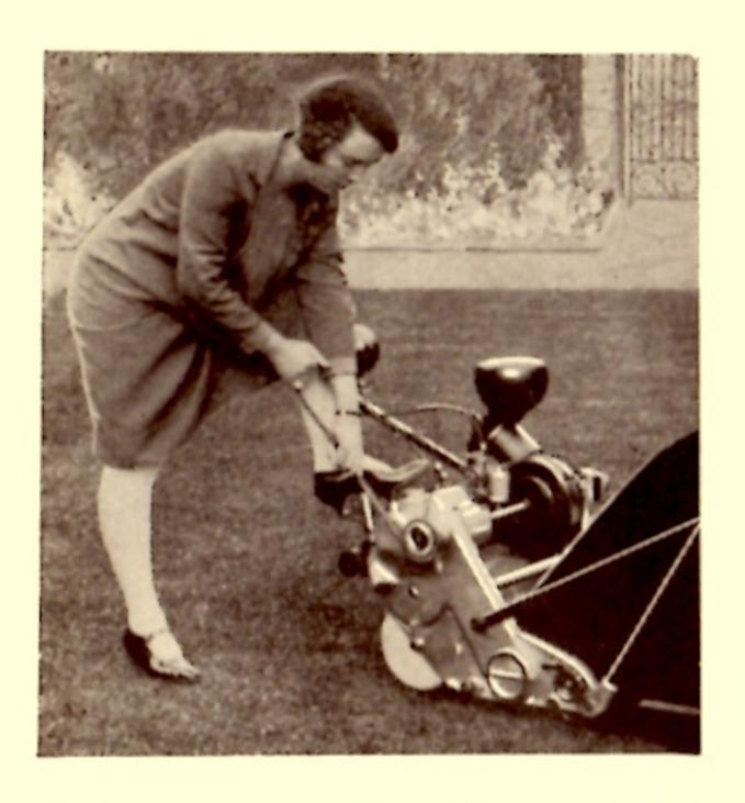
Mowers start by light pressure on "J.P. Super" hand grip lever ("dead man's hand" principle), closing plate clutch. When released the machine stops at once.
